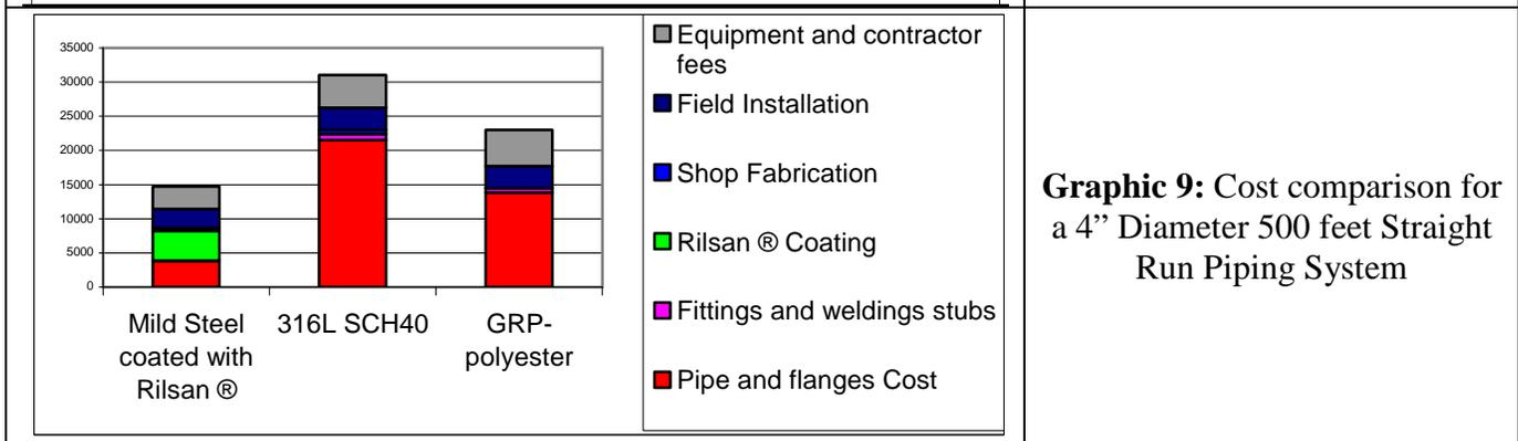
**Graphic 9:** Cost comparison for a 4" Diameter 500 feet Straight Run Piping System
