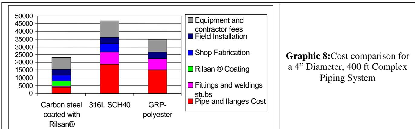
**Graphic 8:** Cost comparison for a 4" Diameter, 400 ft Complex Piping System
