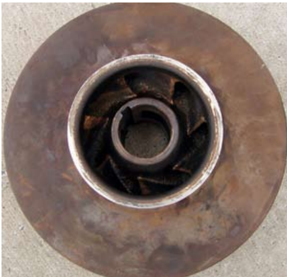
Figure 11. Denise No. 2 impeller prior to the coating process.
