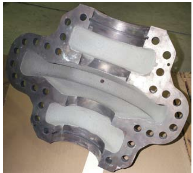
Figure 8. Denise No. 2 horizontal split-case pump – upper half of pump housing after stainless steel plasma coating.
