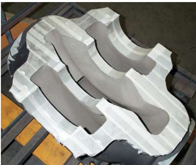
Figure 7. Denise No. 2 horizontal split-case pump – lower half of pump housing after stainless steel plasma coating.
