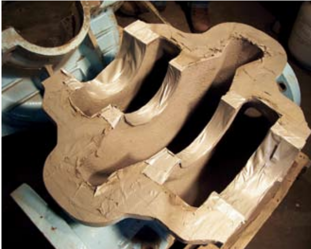
Figure 5. Denise No. 2 horizontal split-case pump – lower half of pump housing after masking the seal areas and grit blast cleaning.
