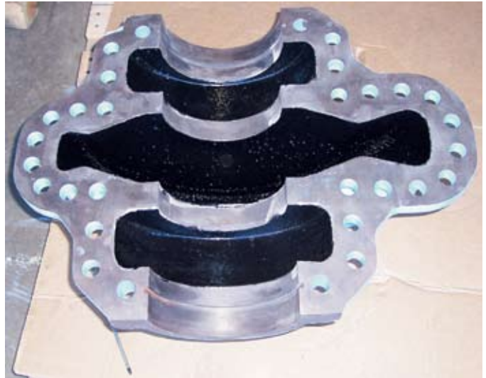
Figure 10 – Denise No. 2 horizontal split-case pump – upper half of pump housing after the application of RILSAN® Fine Powder.
